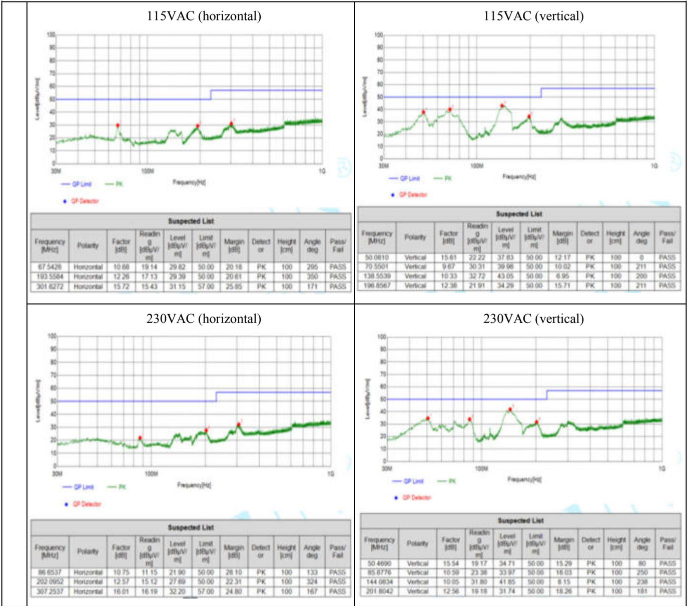
**4.2.4. EMS (EFT: ±4KV, Surge: line to line ±2KV) and EMI (Class B)**
