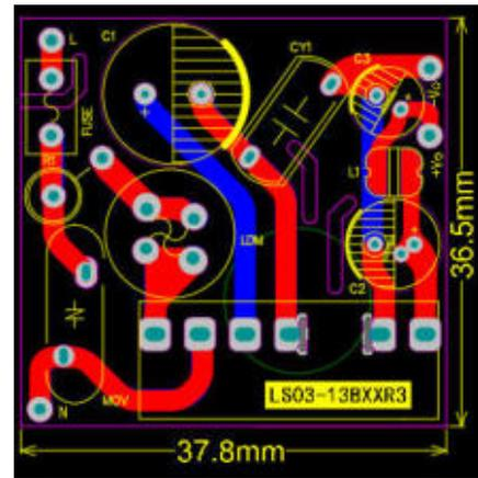
PCB layout (L\*W\*H: 44.0mm\*32.4mm\*23mm)
