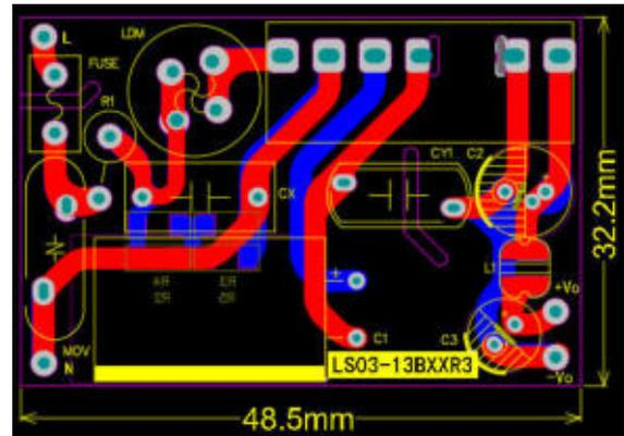
Note: There are three kinds PCB layouts are recommended for this solution. The first is for strict height requirement situations, and the second is for situations where length and width are required but the height is less limited. The third is for strict width requirement situations.
