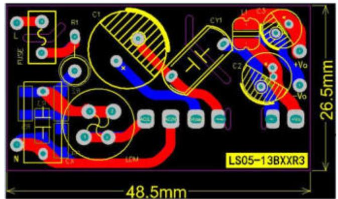
Note: There are three kinds PCB layouts are recommended for this solution. The first is for strict height requirement situations, and the second is for situations where length and width are required but the height is less limited. The third is for strict width requirement situations.
