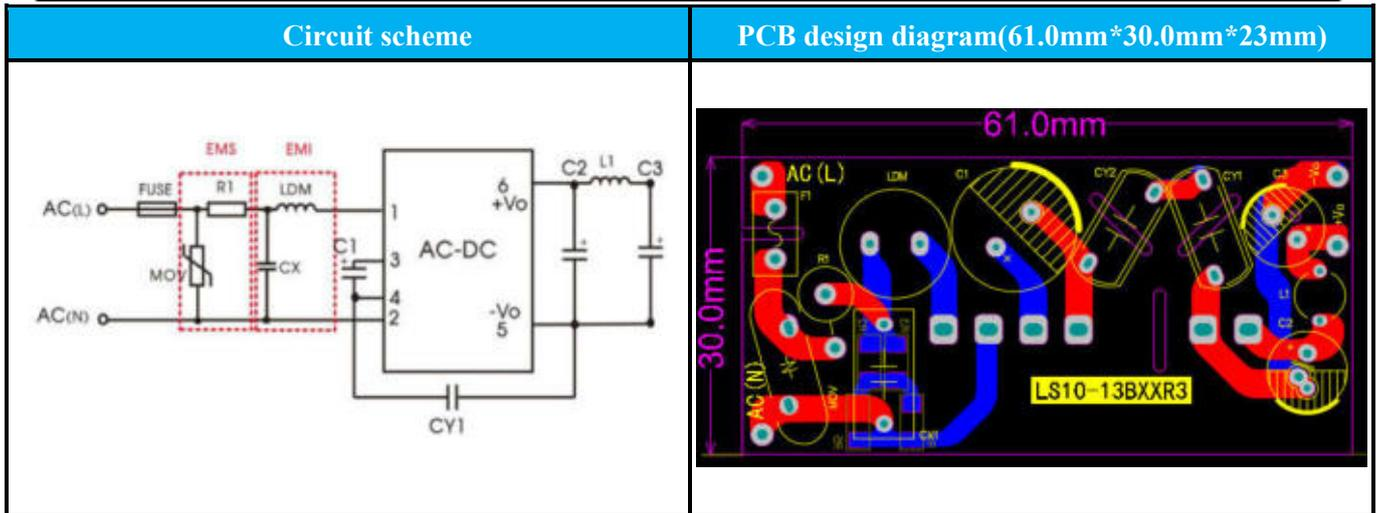
Note: Three PCB layouts are recommended for this solution. The first is to meet the occasions with strict requirements for height, the second is for occasions with requirements for product length and width, and the third is for occasions with strict requirements for width.
