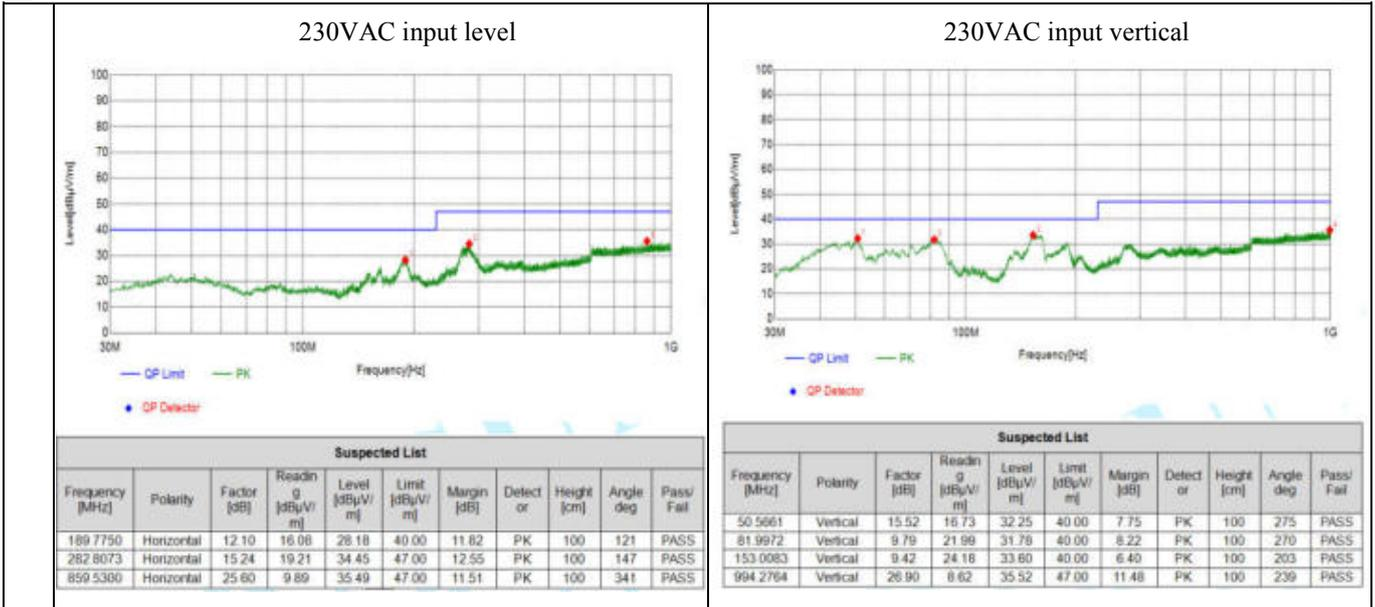
**4.4.5. EMS (EFT: ±4KV, Surge: line to line ±2KV) and EMI (Class B) meets EN60335 standard**
