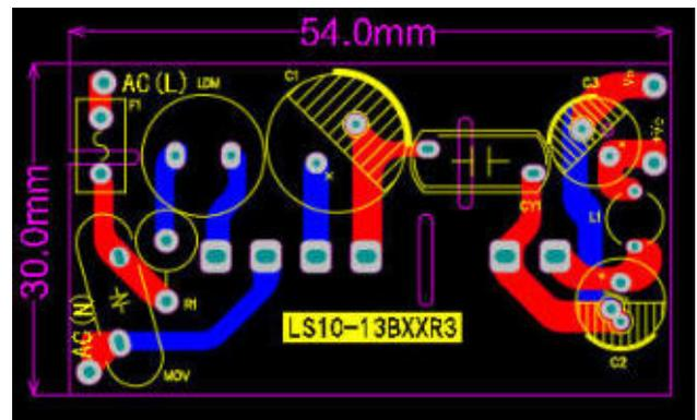
Note: There are three kinds PCB layouts are recommended for this solution. The first is for strict height requirement situations, and the second is for situations where length and width are required but the height is less limited. The third is for strict width requirement situations.
