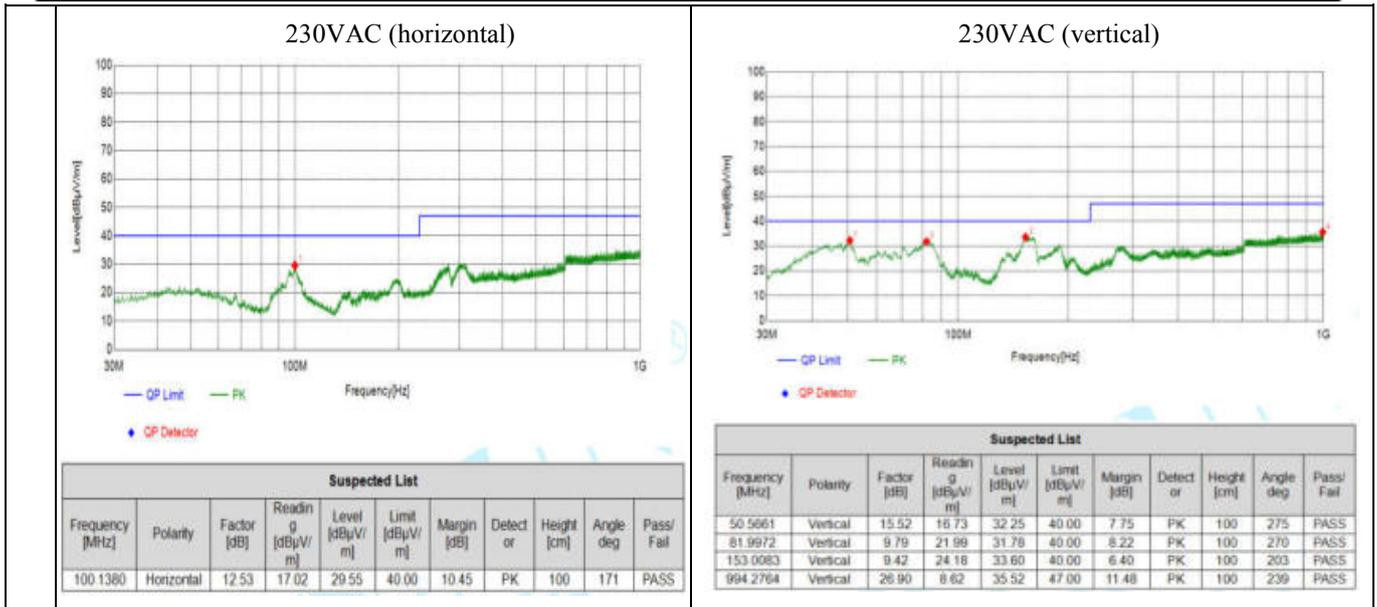
**4.2.3. EMS (EFT: ±4KV, Surge: line to line ±2KV) and EMI (Class A)**
