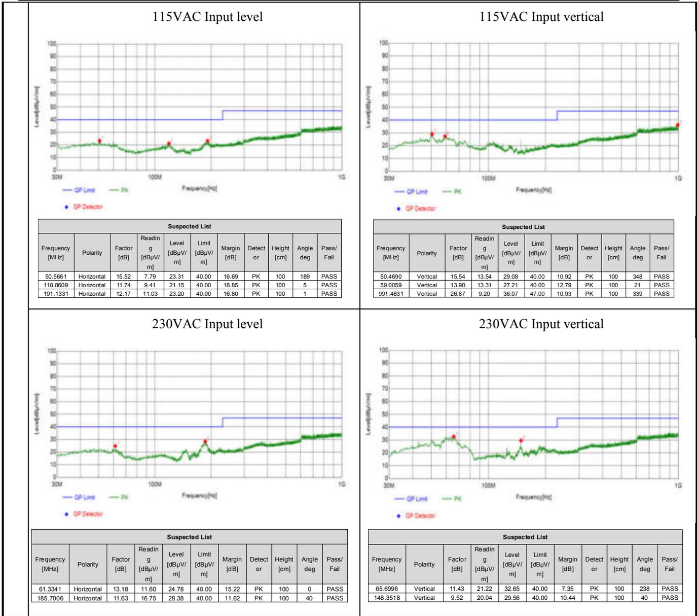
**4.3.5. EMS (EFT: ±4KV, Surge: line to line ±2KV) and EMI (Class B) meets EN60335 standard**
