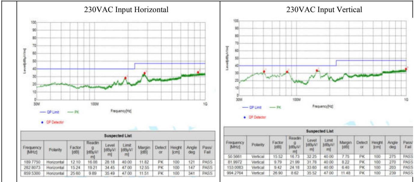
**4.2.5. EMS (EFT: ±4KV, Surge: line to line ±2KV) and EMI (Class B), meets EN60335 standard**
