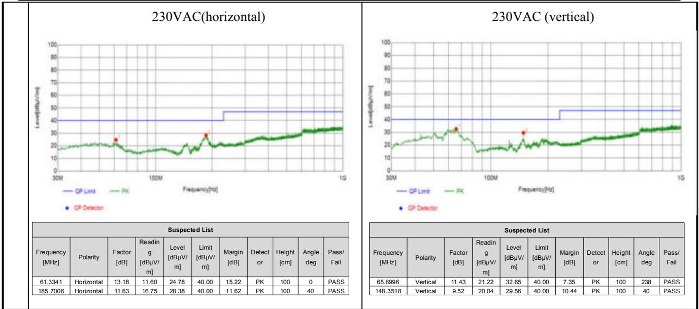
**4.1.5. EMS (EFT: ±4KV, Surge: line to line ±2KV) and EMI (Class B) that meets EN60335**
