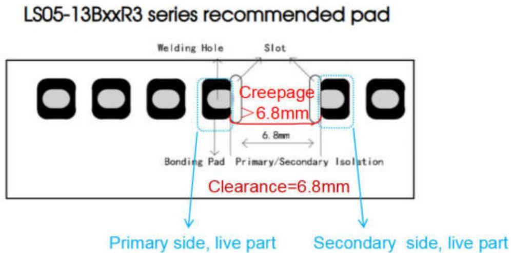
It can be seen from the figure that the electrical clearance refers to the shortest distance between the input terminal and the output terminal, and the creepage distance refers to the shortest distance from the primary terminal to the output terminal after bypassing the slotted hole.
