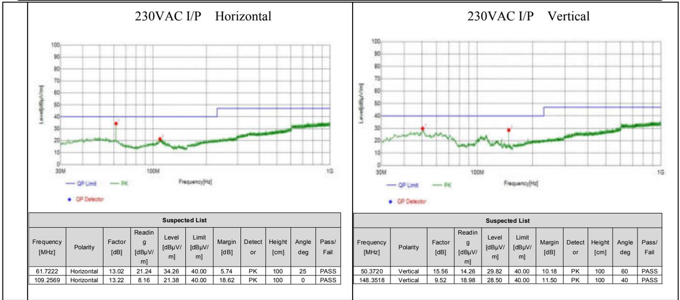
**4.4.3. EMS (EFT: ±4KV, Surge: line to line ±2KV) and EMI (Class A)**
