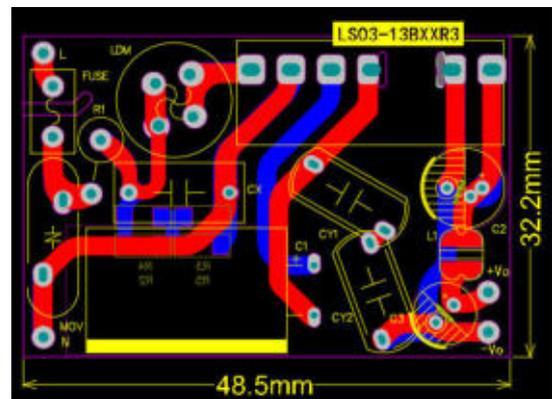
Note: There are three kinds PCB layouts are recommended for this solution. The first is for strict height requirement situations, and the second is for situations where length and width are required but the height is less limited. The third is for strict width requirement situations.
