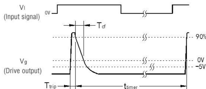
Diagram 16: Definitions of short-circuit detection time delay, soft turn-off time and protection reset time
