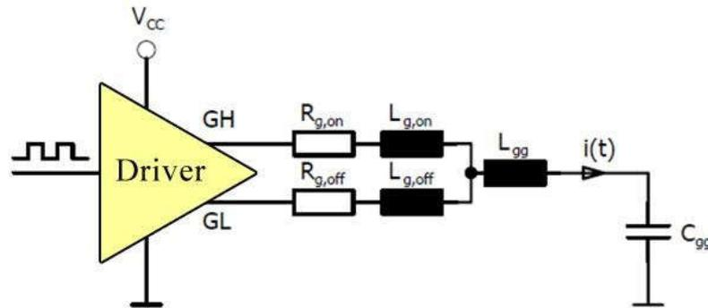
Diagram 10: Typical IGBT Gate Drive Model
