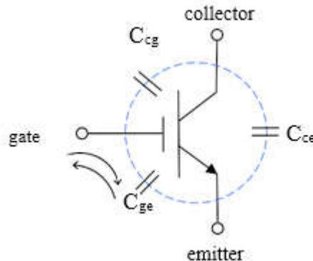
**Diagram 1: Charging and Discharging Model of IGBT Gate**
