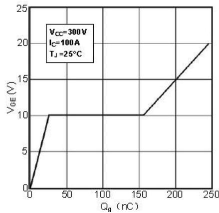
**Diagram 13: Example of IGBT gate C/V changes**
