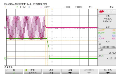
Vin=230VAC Full load shutdown (46ms)
