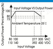
Note: 1.With an AC input voltage between 80 - 100VAC/277 - 305VAC and a DC input between 100 - 140VDC/392 - 430VDC the output power must be derated as per the temperature derating curves;
